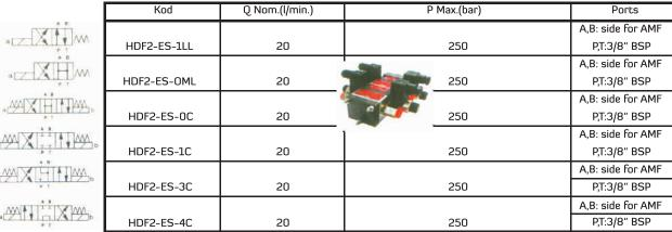
To be combined with function modules AMF (A,B ports on side, top plugged)
